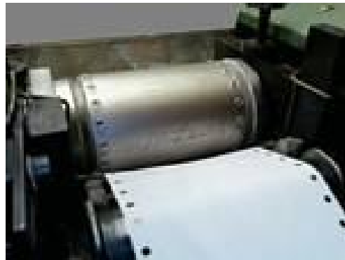
Tractor holes punched under high pressure and waste removed.
